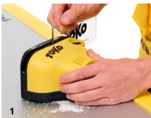
ill. 2) Nordic ski. Expose the centre groove with the Groove Pin Nordic.
