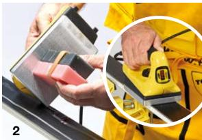
ill. 3) Iron in the wax. Push or pull the iron over the gliding surface. If the iron does not glide smoothly, drip on a little more wax.
