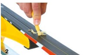
ill. 3) Strip the wax. After about 30 minutes, use the Plexi blade to strip the base in the direction of travel.
